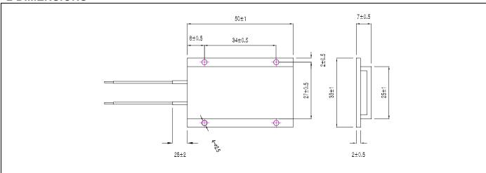
\*Lead wire pipe : Plastic Ø1.5, Length 25±2mm
