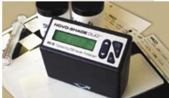
The Novo-Shade Duo will quickly and accurately calculate the opacity of a coating applied on a Leneta type chart
